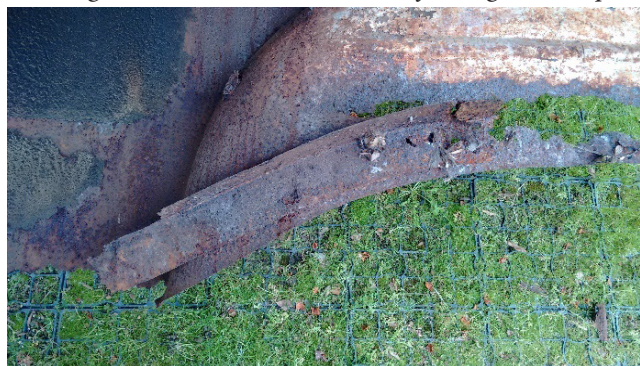
Fig. 3 - RIGHT What remained of the right rocker panel
