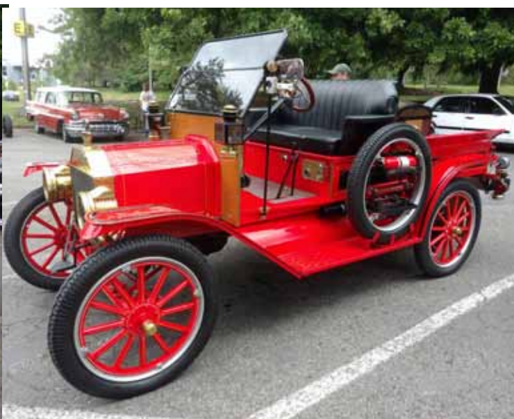
Model T with an 10" wheel driving a outboard alternator
