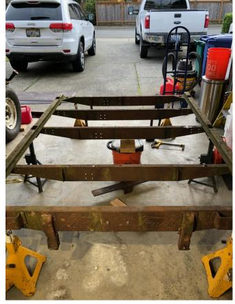
This is the new length. 84 inches exactly on both sides. Now I need to do some work to ensure proper alignment before welding.
