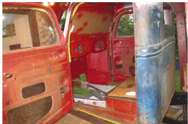
Interior and frame get some paint.
